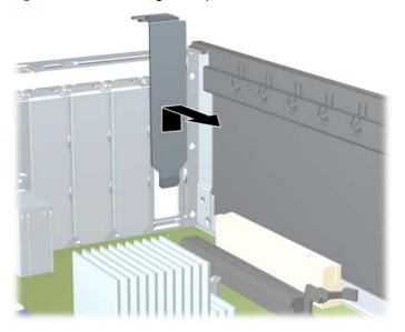
Figure 6-18 Removing an Expansion Slot Cover
